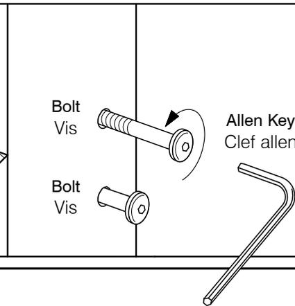
**BOLT AND BARREL NUT ASSEMBLY SYSTEM**
