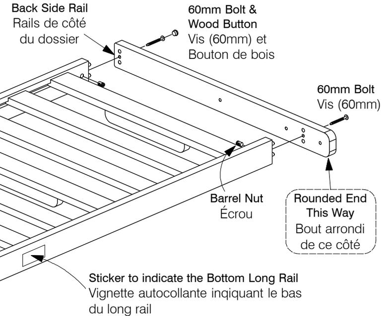
After tightening all the bolts on Seat Deck, push fit or lightly tap the Wood Buttons into the holes as shown.
