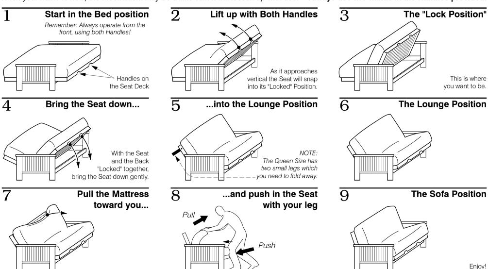
$<sup>^</sup>st$ Please Note: If the rollers of the mechanism become improperly disengaged, the Back Deck could come down more quickly than you expect!
